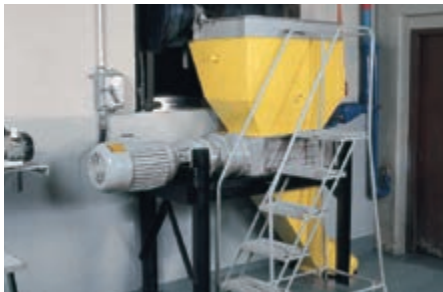
4-SHRED-H with Custom Hopper and Discharge Chute
